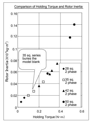
Fig. 6 Holding Torque – Rotor Inertia Chart
