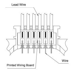
Fig. 3 Conventional Lead Wire Connection
