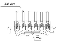
Fig. 4 Lead Connection of the Developed Product
